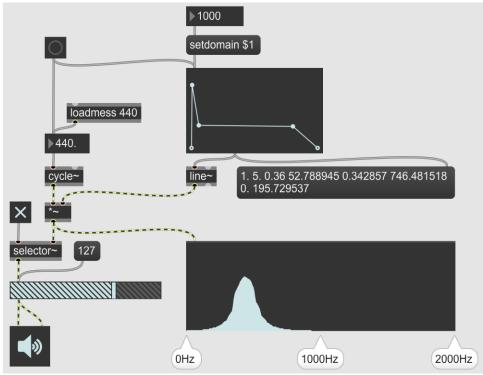
Note that a bang message is required to trigger the "function" object to send a message to "line~" • Use the "kslider" object to create a MIDI keyboard that you can play with your mouse
