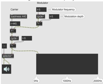
• Use the "kslider" object to allow easy control of the carrier frequency and set the modulator frequency as a specific multiple (doesn't need to be a perfect multiple)
