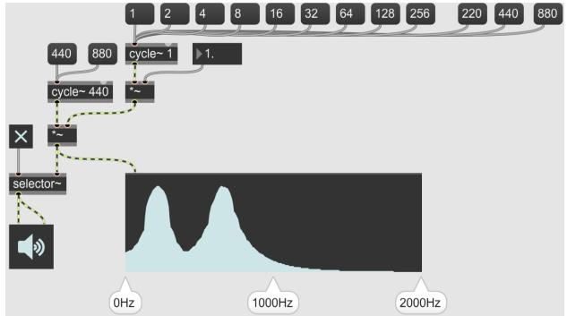
• Above is an example when the carrier is 440Hz and the modulator is 220 Hz, and we see two tones at 220Hz (440Hz – 220Hz) and 660 Hz (440Hz + 220Hz)
