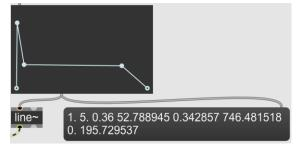
• Use the ADSR envelope to modulate the amplitude of a sinusoid signal
