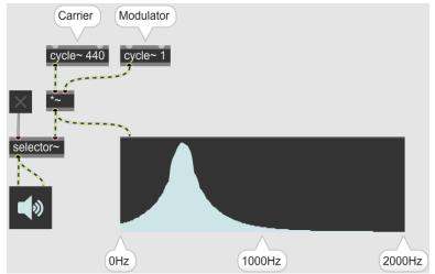
• When the frequency of the modulator signal is high, it actually creates a separate tone of its own
