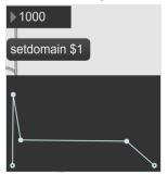
• Use a "line~" object connected to the second outlet of the "function" object, which outputs a series of numbers that describes the function
